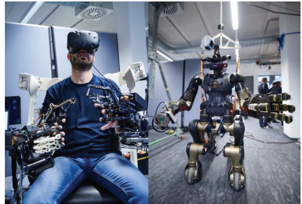
Figure 6. Tele-operated robot Centauro can fulfil tasks such as climbing stairs, navigating obstacles and using power tools. Image Credit -© Volker Lannert/ Uni Bonn [21].
